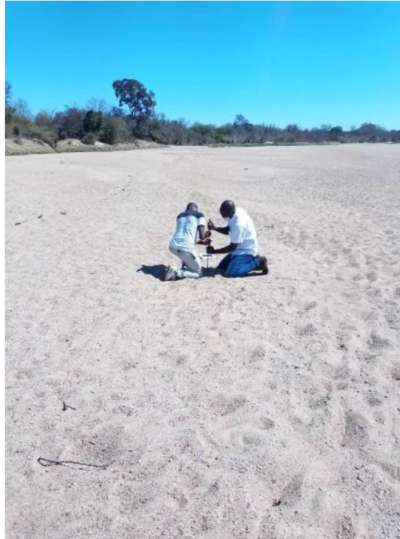
Fig. 3: Sand probing indicated depths of >3m. According to Hussey (2003) sections with depths greater than 3m are good for sand abstraction
